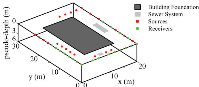
**Figure 1** 3D scheme of the surface sources and receivers distribution. The foundation footing is highlighted in dark gray, while locations of some parts of the sewer system are highlighted in light gray. The source receiver's distribution was optimized to investigate the corner of the building closest to the axis origin while the entire perimeter was injected.
