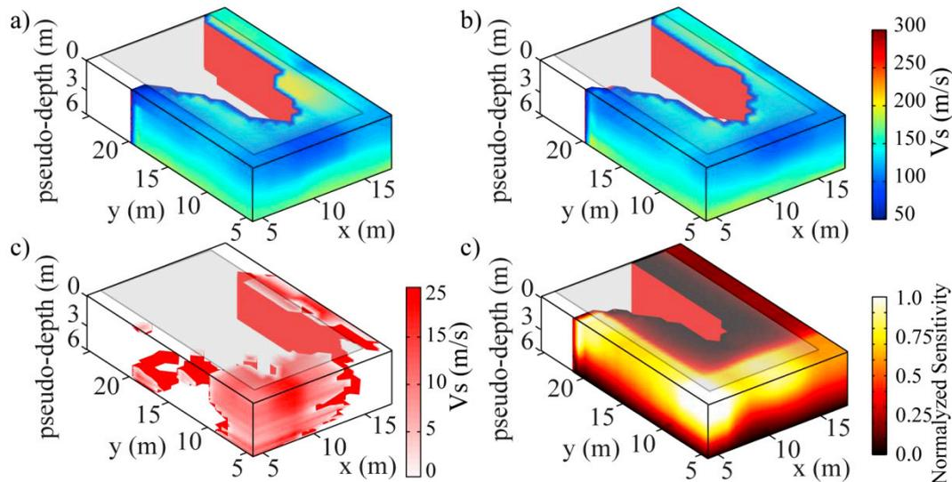
**Figure 3** Apparent  $V_S$  (a) before and (b) after the resin injection. c) Stiffening effect in term of percent increase of  $V_S$ . d) Normalized sensitivity accounting for the reliability of the results. Portions of the model for which to retrieve any result was not possible with the present sources-receivers configuration are not colored. The footprint of the building is highlighted with the gray rectangle.
