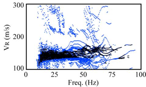
**Figure 2** An example of the SASW-like cloud of points in the  $f$ - $V_R$  domain. In this example, the blue points are filtered out while the black points are those which comply with eq. 2.
