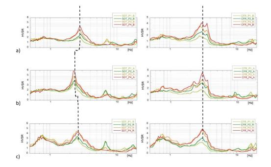
Figure 6 – HVNSR spectra acquired on STD side (left) and CFR side (right): a) before the earthquake; b) after the earthquake; c) after the damage repair.
