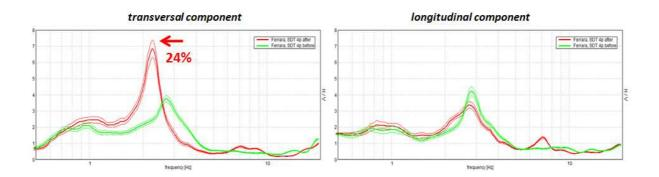
Figure 7 – HVNSRs acquired on STD side for the transversal component (left) and for the longitudinal component (right), before the earthquake (green line) and after the earthquake (red line).
